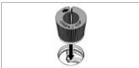
Fig. 9.8 How to insert the odour filter through the extractor opening
