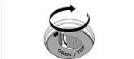
Fig. 9.9 How to place the odour filter in the end position
