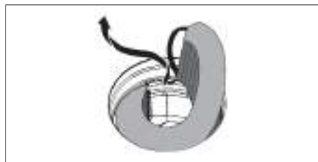
Fig. 9.6 How to remove the odour filter through the inlet opening
